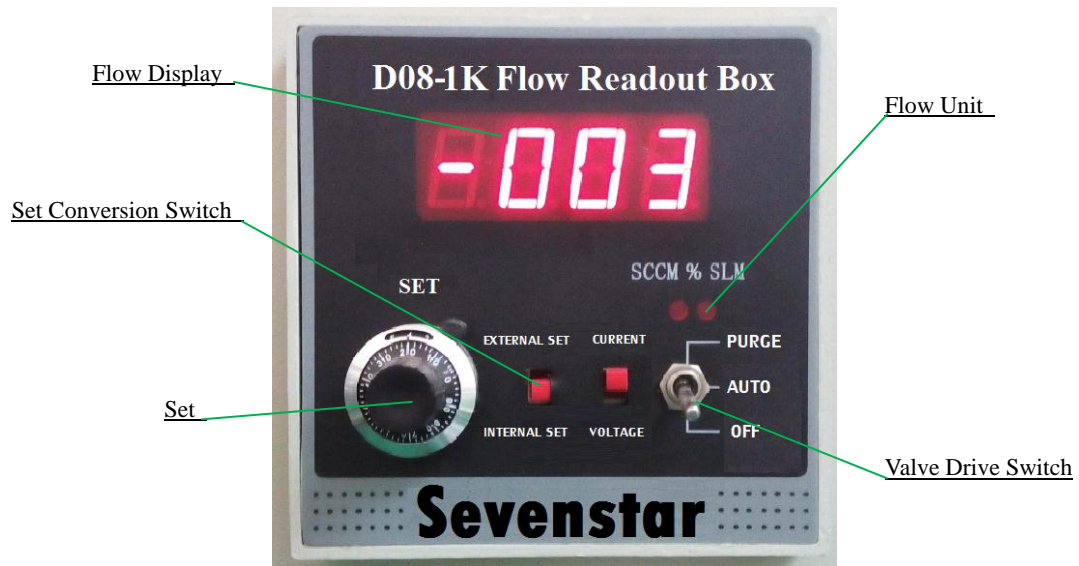
Figure 10. Flow Readout Box Operating Panel
