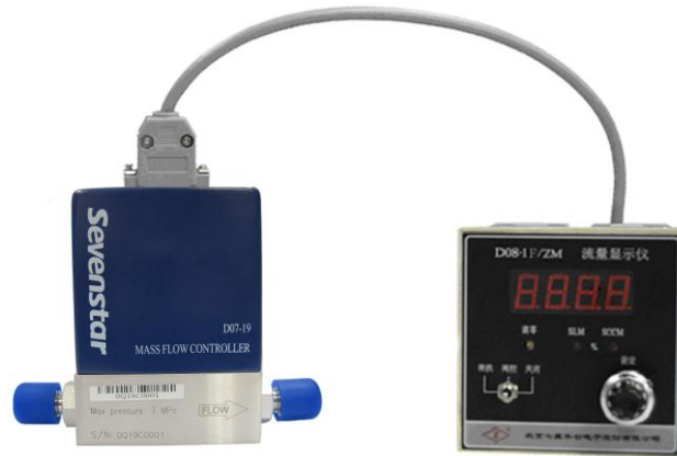
Figure 1. D07 –19C MFC and Readout Box
